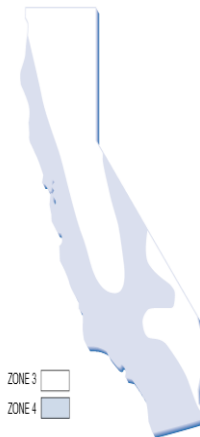
Figure 9—Seismic zones in California. All of California is in seismic zone 3 or 4 on U.S. Geological Survey maps. There are four zones; the higher the number the higher the earthquake danger. Stronger standards for buildings in zones 3 and 4 have been adopted in the Uniform Building Code.
